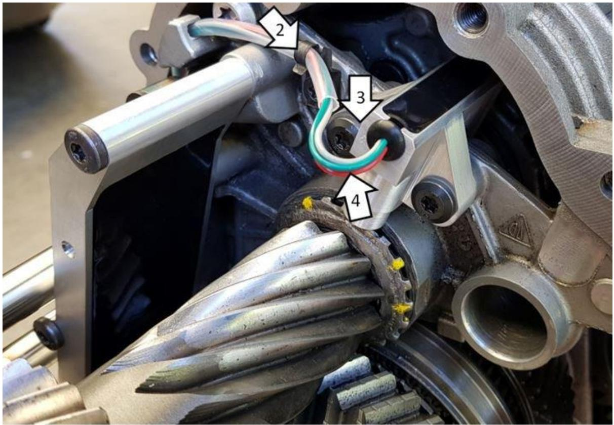
Ensure the bend radius is not too tight where the wires exit the speed sensor.
