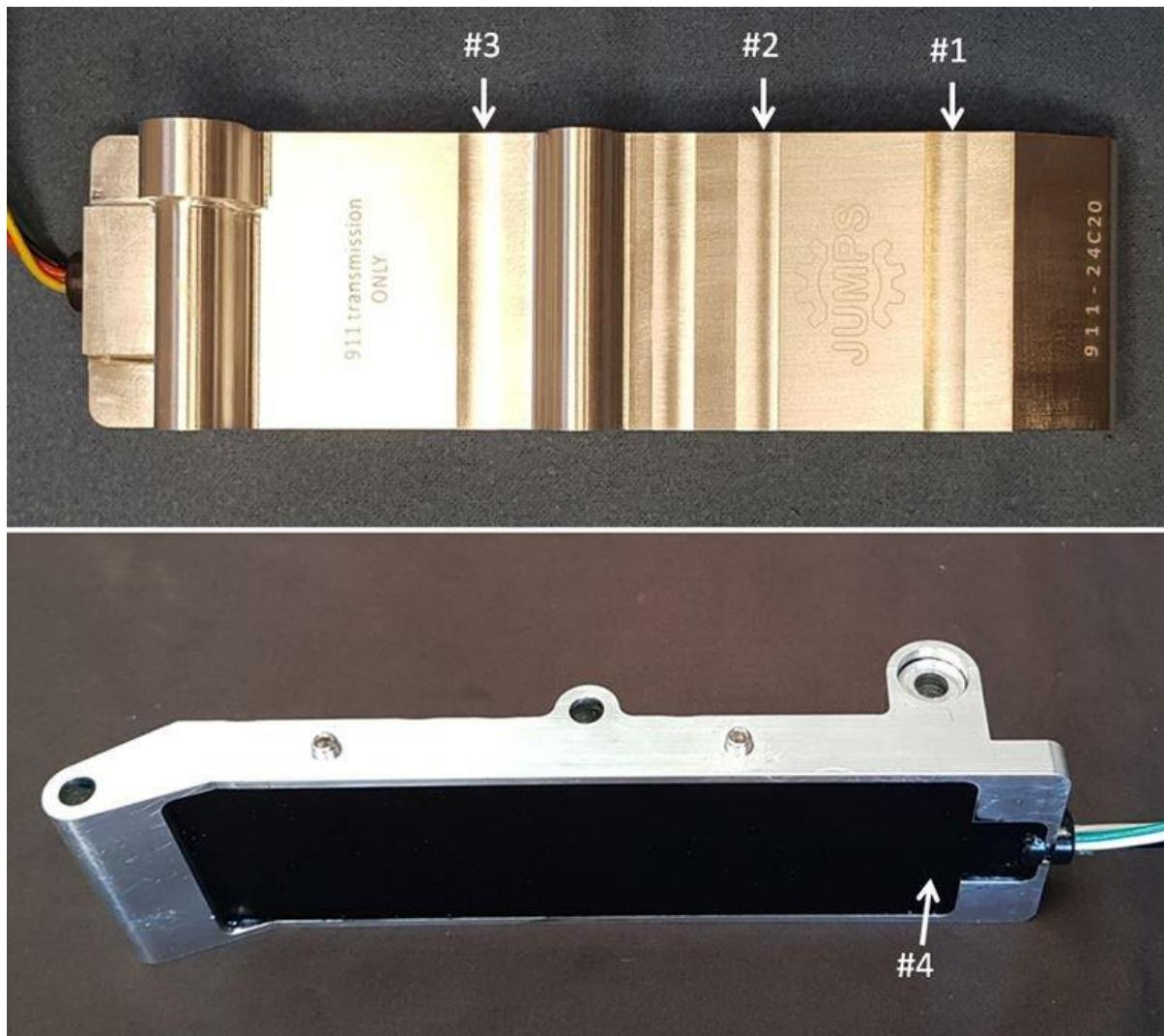
3) After installing the sensor, but before putting the case back on, connect PIWIS and display the Shift Rod actual values. All four distance sensor channels should read less than 1.5mm (+ or -) with all four shift rods in the central position.
